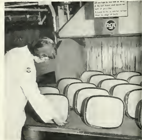
The tubes move slowly through an oven where the fluorescent screen surface is baked.
