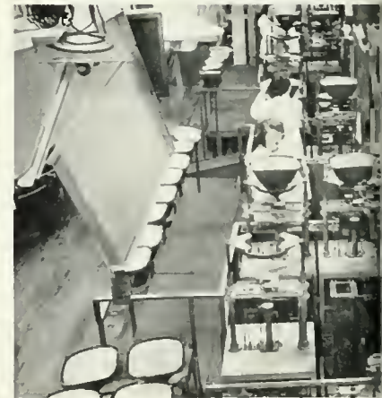
Tubes are cleared of air by pumps which create the vacuum required for television kinescopes.
